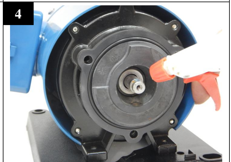
Spray water on the shaft as lubrication.
