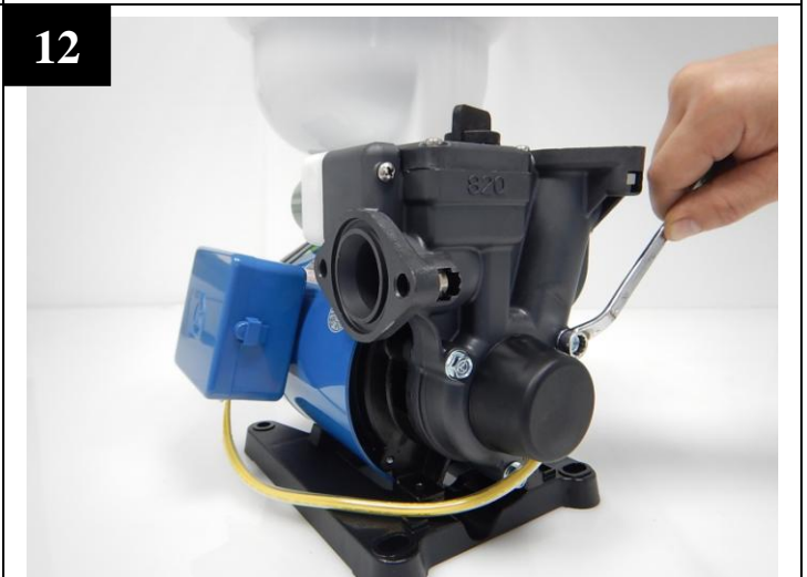
Install the pump casing and using wrench to tighten up the stud bolts. ※Torque 50-60 kgf · cm
